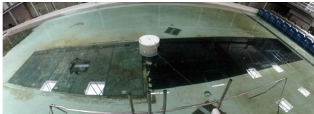
Figure 5: The cylindrical floater experimental case Moura Paredes et al. (2016); Palm et al. (2016) used for the validation of the rigid motion solver.
